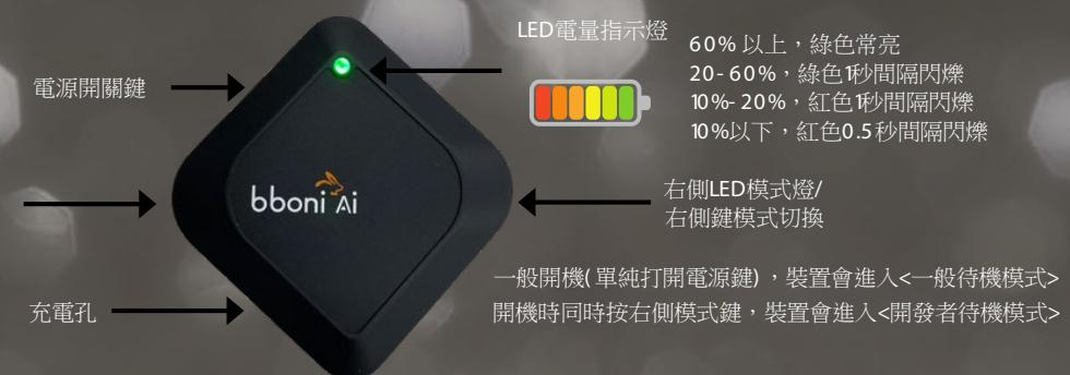
The device displays the charging indicator lights **only when powered on**. In connected mode, developers can control the **color and blinking pattern of three LEDs**, enabling rich and customizable feedback effects.
